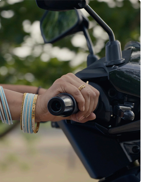
Magic Twist™ allows the rider to decelerate using the throttle itself and minimise the use of brakes.
