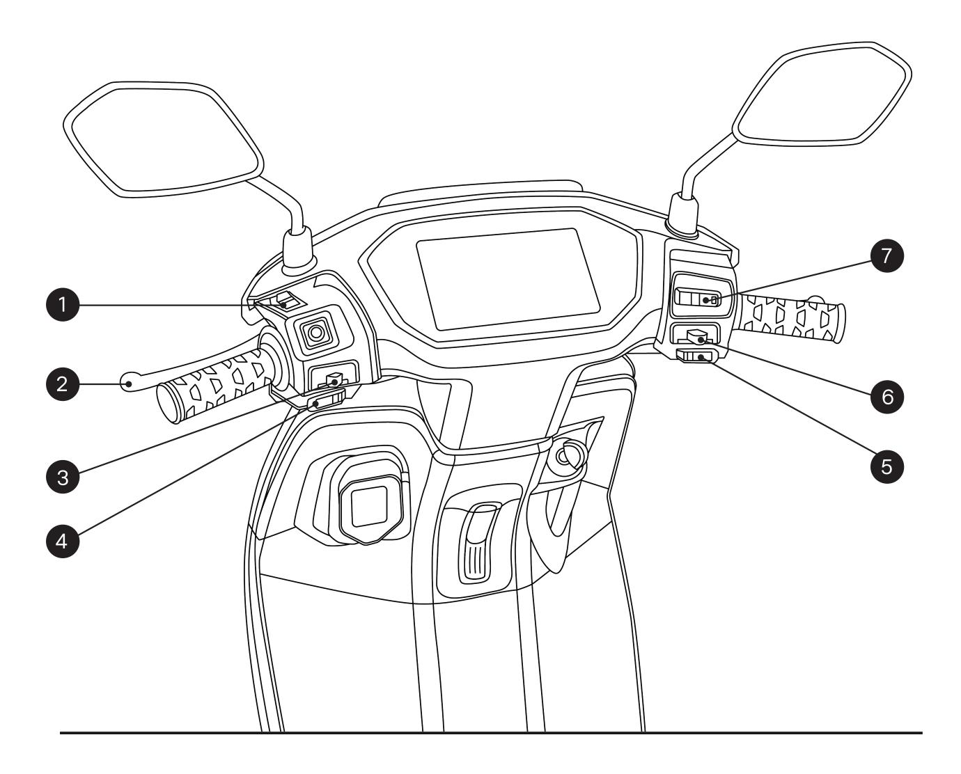
1 Headlight high/low beam switch 5 Motor starter
